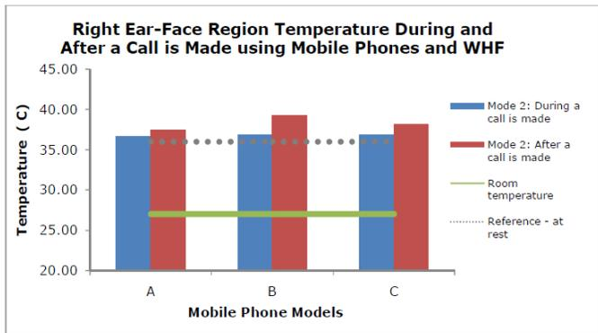
Figure 5 Right ear-face region temperature for during and after a call is made for Mode 2
