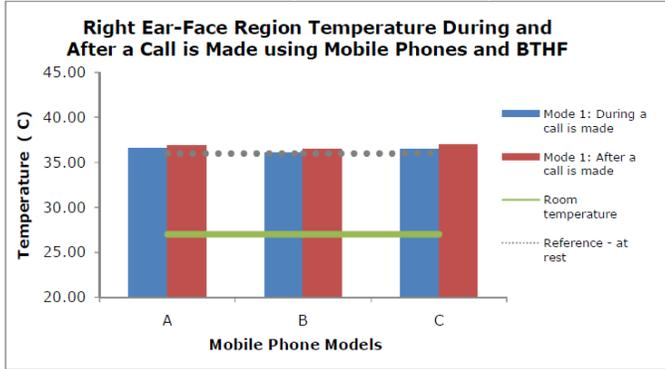
Figure 4 Right ear-face region temperature for during and after a call is made for Mode 1
